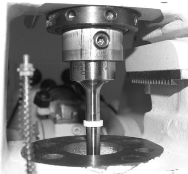
Fig. 2. Measurement setup used in US transmission measurements with instrumented punches.
